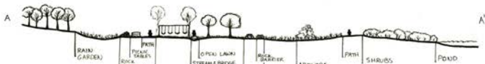
Section A-A' A section taken of the play space, looking north. Seating on both sides of the play space provides parents a place to watch their children. Rock barriers between seating and rain gardens allow for closeness but maintains safety.
