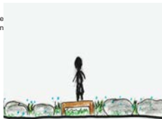
Section Cut B-B' This section shows the raised boardwalk in relation to the boulders.
